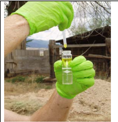
Figure 12. HACH™ Test for dissolved sulfide (courtesy of ESN Rocky Mountain).
