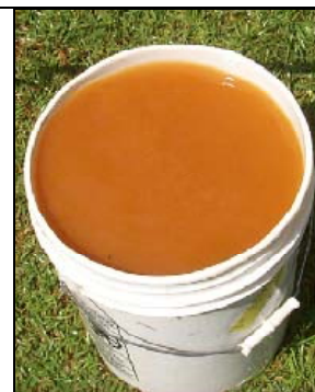
Figure 10. IRB (Gallionella sp.) and particulate ferric iron account for the orange color and “metallic” odor and taste.
