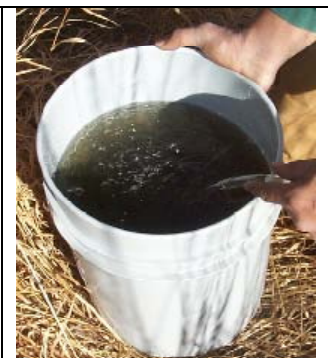
Figure 11. Strongly reducing environment with SRB yielding smell of “rotten eggs” and color due to dissolved ferrous iron sulfide.
