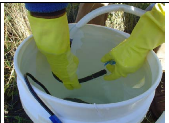
Figure 4. Collecting a water sample in a 40 ml VOA for dissolved methane analysis. A 250 ml bottle is preferable for dissolved hydrocarbon analysis.
