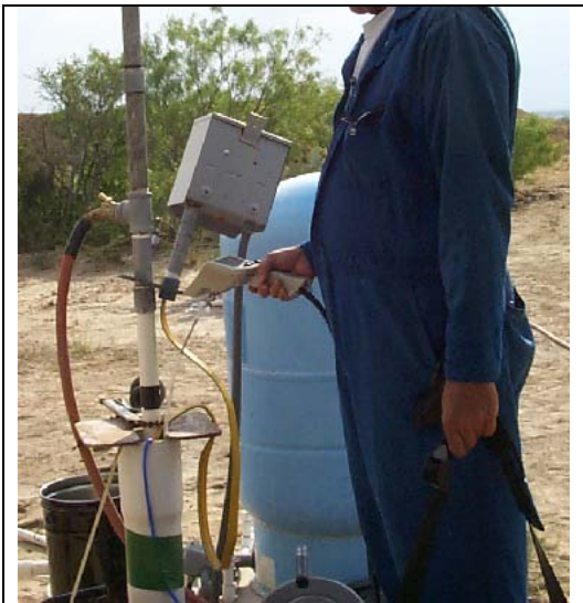
Figure 3. Field technician using a portable flame ionization detector to monitor well head gas while purging a well.
