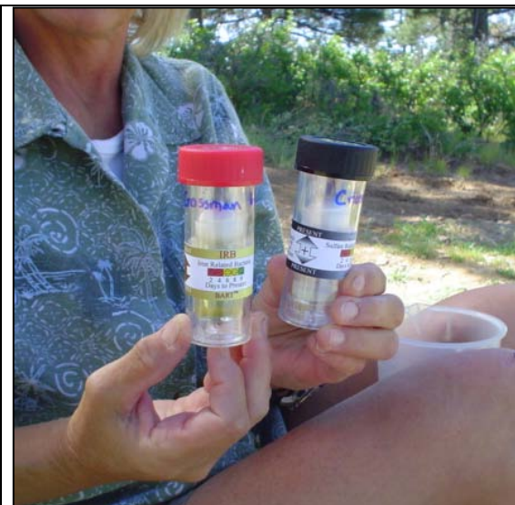
Figure 6. BART sample vials: IRB- red cap; SRB black cap (photo courtesy of Four Corners Geoscience.
