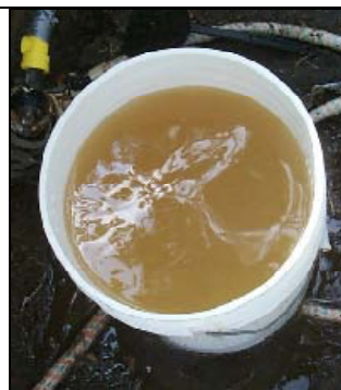
Figure 9. Murky water with odor like sewage indicative of enteric bacteria.
