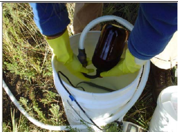
Figure 5. Filling a 1-L Boston round bottle with water for extraction and analysis of dissolved hydrocarbons.
